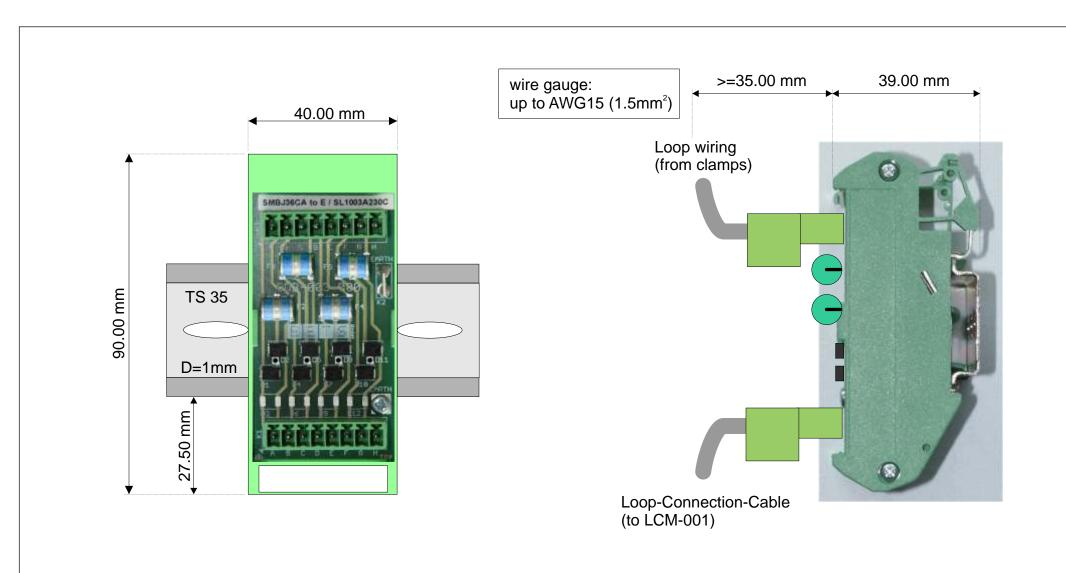
Frontview of COB-003 for DIN rail mount (rail 35mm x 7.5mm, size 1mm)
